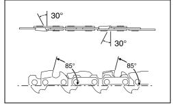
All cutters must be sharpened to the same angle, 30°. Different angles result in a roughly, irregularly running chain, increase wear and tear and cause chain beakage.
